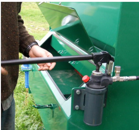
Hydraulic pump for hopper lid
